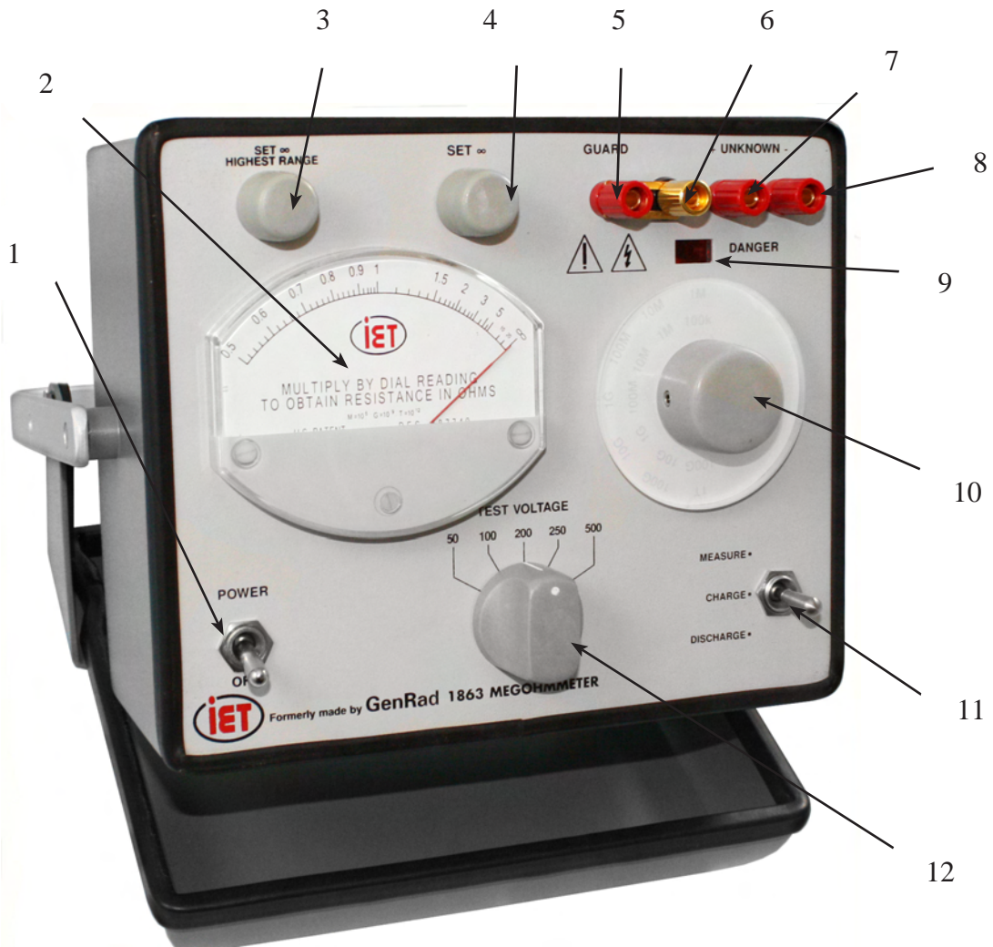
Figure 1-2. Type 1863 Front-panel Controls, Connectors and Indicators
